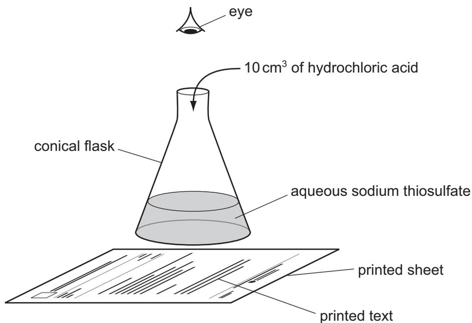
A student used this method to investigate the effect of changing the concentration of the sodium thiosulfate solution on the speed of the reaction. The student used different concentrations of sodium thiosulfate solution. All other variables were kept the same.
